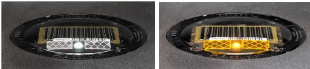
Figure 4;6: Astucia 1 candela white and amber stud conspicuity comparison
